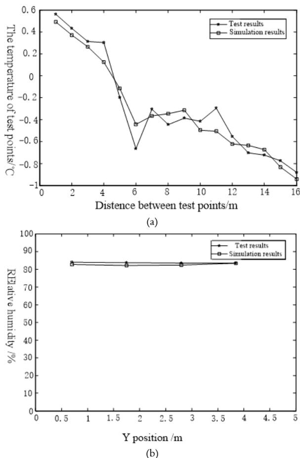
**Fig. 3.** (a) Validation of temperature distribution; (b) Validation of relative humidity distribution
