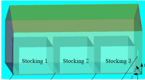
**Fig. 2.** The computational domain of citrus ventilation storage
