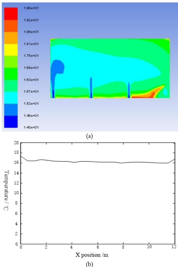
**Fig. 5.** (a) Temperature contour of Y=3.5 m section; (b) Temperature curve of X section
