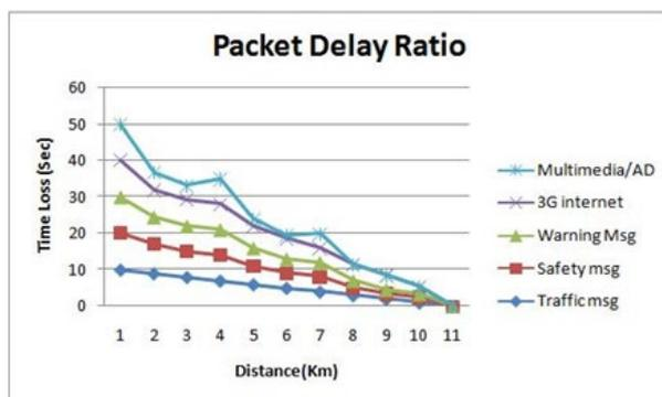
Fig. 8. Packet Delay Ratio
