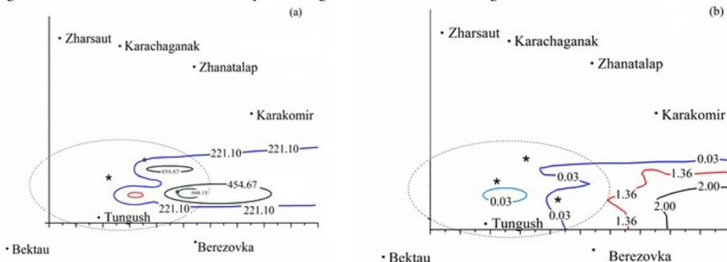
**Fig. 6.** Isograms of NO<sub>2</sub> concentration in percentage of TLV a) at 70 m height; max NO<sub>2</sub> – 921.63, b) at 80 m height; max NO<sub>2</sub> – 2.82
