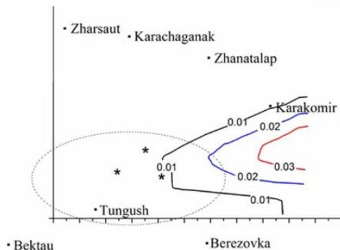
**Fig. 3.** Isograms of CO<sub>2</sub> concentration in percentage of TLV at 70 m height, max CO<sub>2</sub> – 0.03
