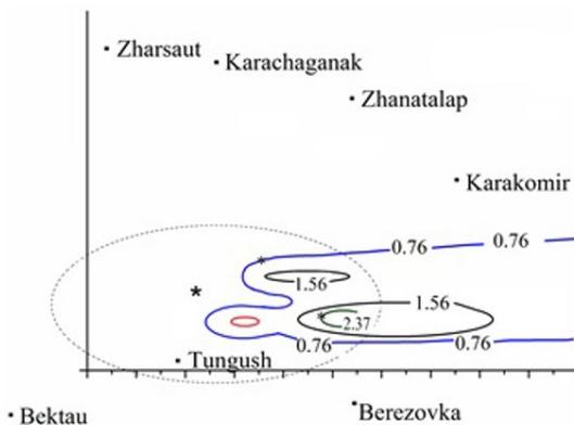
**Fig. 5.** Isograms of CO<sub>2</sub> concentration in percentage of TLV at 70 m height; max CO<sub>2</sub> – 3.17
