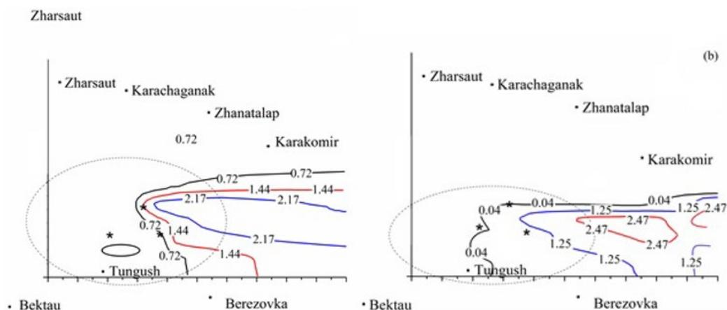
**Fig. 2.** Isograms of CO<sub>2</sub> concentration in percentage of TLV at 10 m height, a) max CO<sub>2</sub> – 2.89, b) max CO<sub>2</sub> – 3.69
