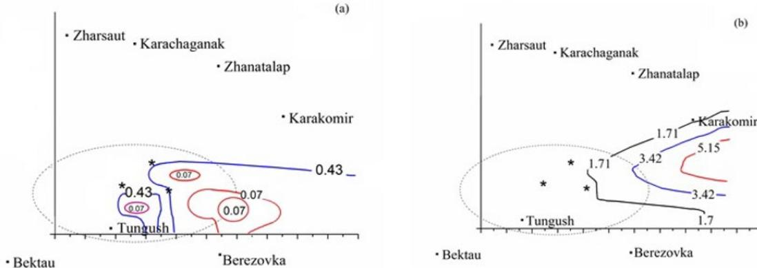
**Fig. 4.** Isograms of NO<sub>2</sub> concentration in percentage of TLV a) at 10 m height; max NO<sub>2</sub>– 1.75, b) at 80 m height; max NO<sub>2</sub>– 6.85
