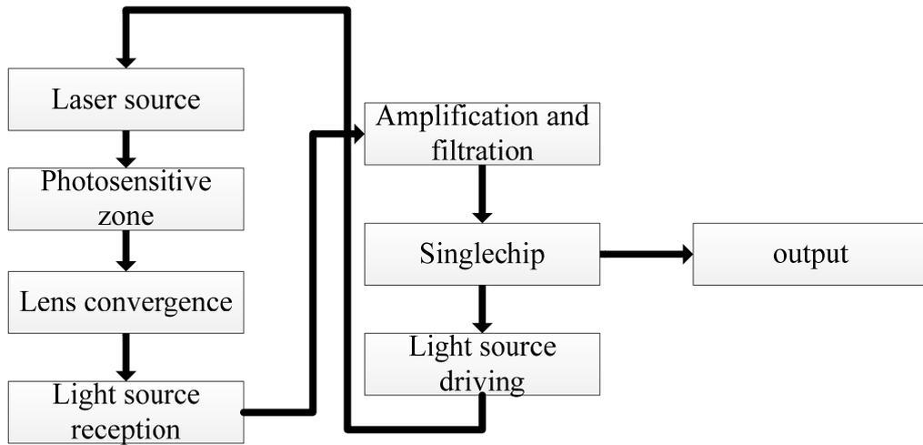
**Figure 2 Information acquisition module for environmental pollution area**
